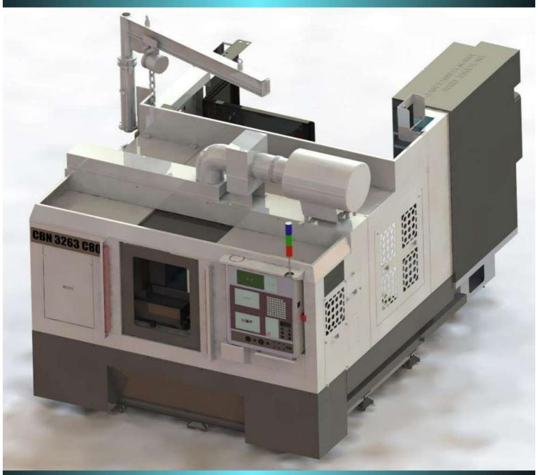
CSG-3263 has been specifically developed to meet the high quality and productivity demands of Cam-lobe grinding operations using CBN grinding wheels
